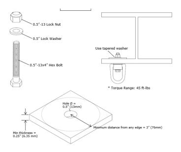
**IMPORTANT:** Use a grade 10.9, grade 12.9 (or equivalent) bolt no shorter than 4" (100mm) with a locking nut and washer in steel applications. When installed, the swivel anchor must be flush with the steel surface.
