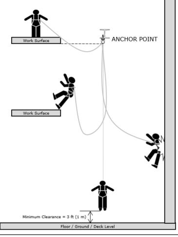
• The maximum dynamic forces exerted on the user during a fall arrest must be limited to a maximum of 8kN (1800 lbf). In the EU, these forces must be limited to 6 kN (1,350-lbf) for N-8232100.
