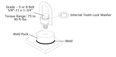
**IMPORTANT:** Before installation and use, the welding procedure must be approved by a competent engineer or other qualified person. Specifically, that the welding procedure is compatible with any and all structural & operational characteristic of the selected installation location.
